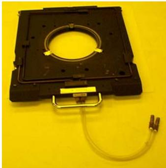
4.3.2 Modified mask holder for 7-inch glass, for contact mode only on 4 and 6 inch wafers.
